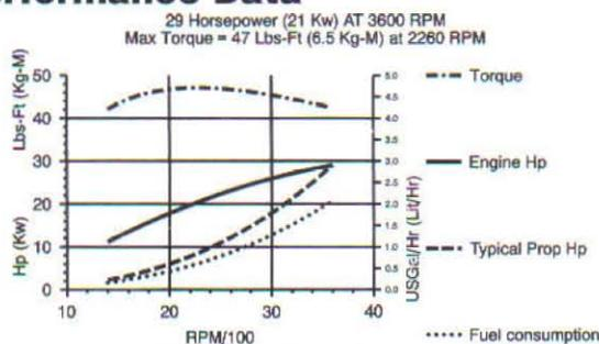
Westerbeke recommends a propeller that will allow the engine to turn 3500-3600 RPM underway at full throttle
